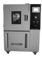
**Ozone Test chamber** is used for testing rubber and polymer. Put the sample in certain density ozone environment, after having certain discoloration or the scheduled time and compare with the standard card. Applications of Ozone Test Chamber
